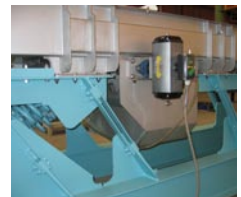
Mass-compensated feeding conveyor FSM – 60 m long – for the food industry with product distribution system (right).
