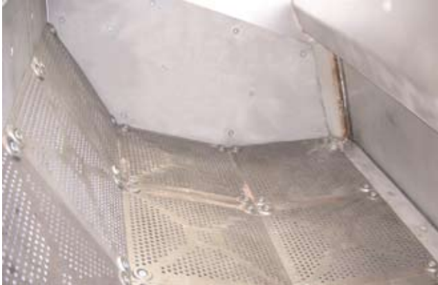
Attrition sink made of modular highly wear-resistant hart cast iron perforated plates
