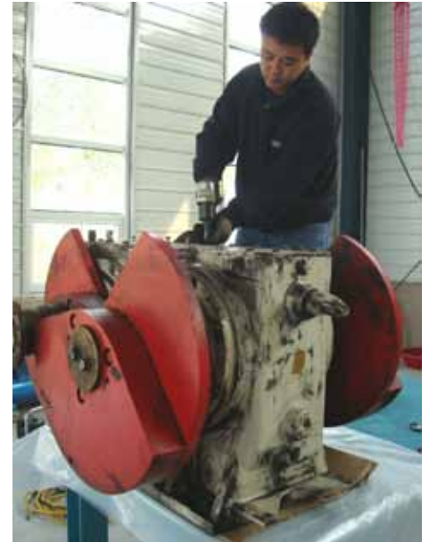
Employee repairing an excitor
