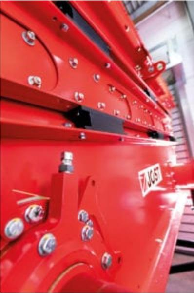
*Optimized lateral sealing between mats and screening body at a maximized usable width*
