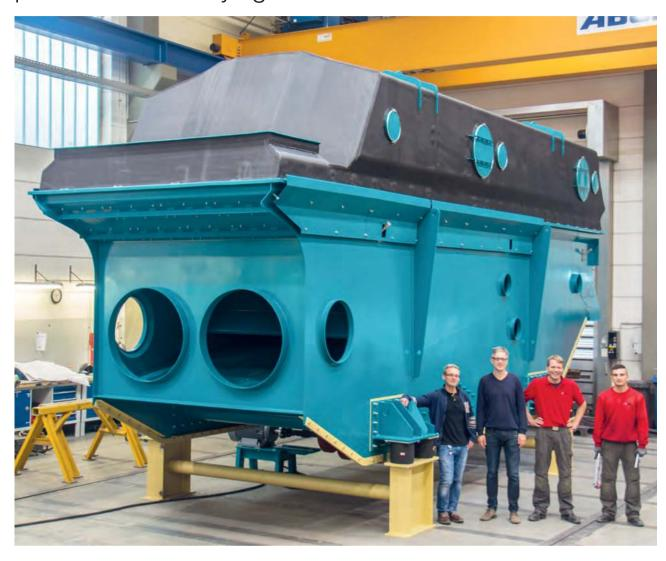
JOEST vibrating fluid bed dryers for bulk materials transfer the heat energy required for drying by convection, i.e. via direct heat transfer, so that the heat transfer medium comes directly into contact with the product. The heat transfer is typically performed using temperature-controlled warm or hot air. A subdivision into different zones for drying and cooling is possible.
