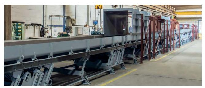
The JOEST Vibrating FSM Trough Type Feeder for European customers will be used for the evacuation of burned slag to an ash bunker. This feeder will be positioned beneath two waste incineration furnaces.
