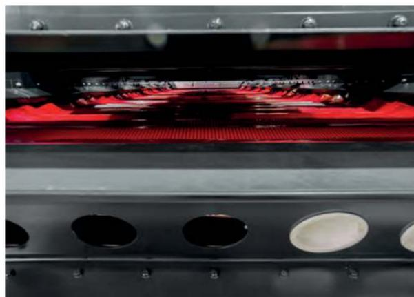
In March 2016 JOEST delivered one of the biggest OSCILLA screens so far. The JOEST flip-flow-screen OSCILLA is the ideal solution for sticky and difficult to screen materials with a typically particle size between 0 - 100 mm (0 - 4 inches).
