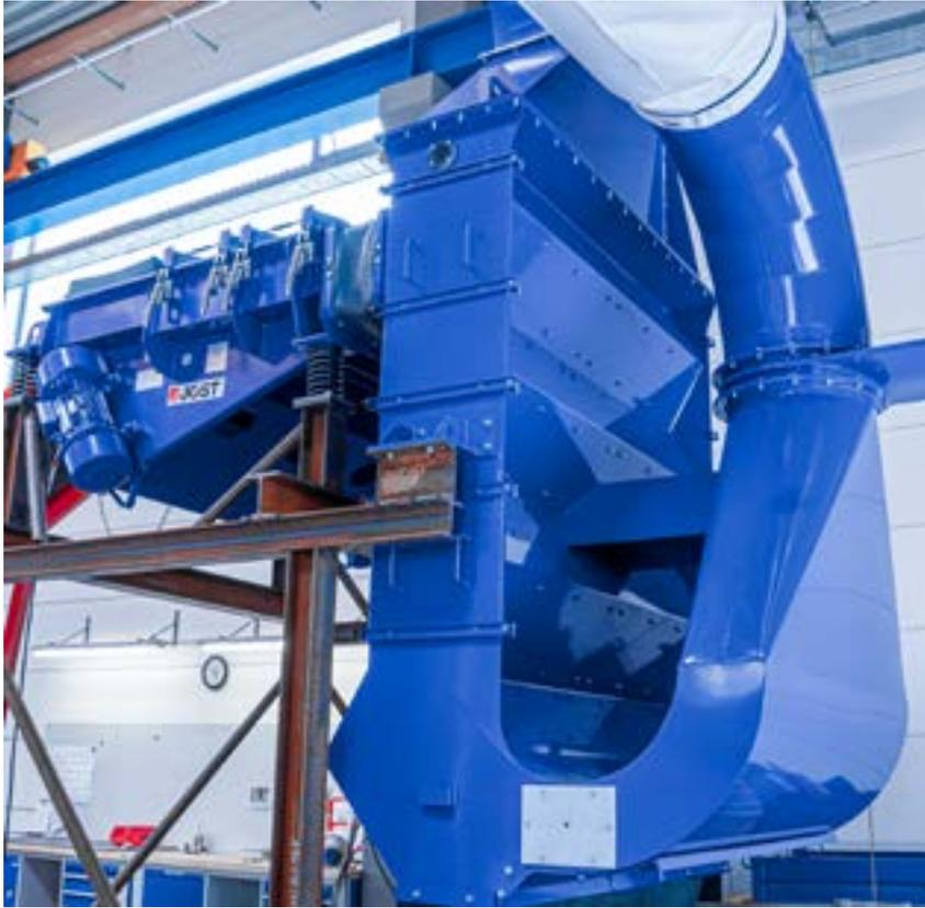
*Sifting and sorting:* ▲ beams also feature special profiles to ensure flexibility and efficiency. They are simply cut to the desired length and bolted to the machine body.
