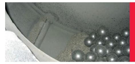
Usually, dross consists of approximately 40-60% metal and 60-40% oxide. The objective of such a plant is to separate the metal from the oxide, to retrieve the metal as pure as possible and to dispose the oxide as waste. The oxide portion is also referred to as slag or dross.
