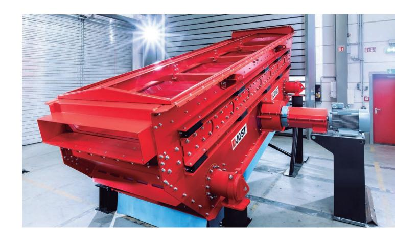
tions with extremely high acceleration values. Additionally, the screening mats are installed very high up at the end of the cross bars to ensure an optimal sealing to the sides while simultaneously ensuring a maximal effective width. The combination of operational safety and efficiency of the useable classifying surface is another JOEST feature.
