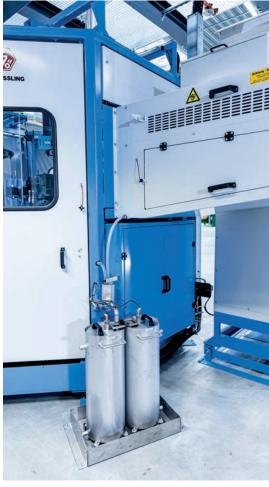
lled. Since 95% of the oil sticking to the material is separated in the first step, a carryover of oil is avoided. The water purification and automatic refill function enable a long lifetime of the washing solution. All inlets, outlets and pumps of the unit are fitted with filters that col-lect debris such as metal shavings from the fluid circuits. This eliminates causes of damage and significantly reduces maintenance.
