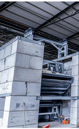
three additional fractions, smaller than 16 mm, 16 to 26 mm and larger than 26 mm are gained.
