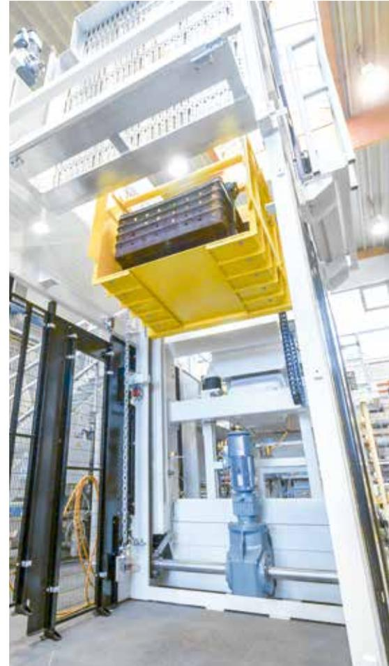
demand formula. During the filling process, the container stands on a vibrating table, resulting in an even parts distribution throughout the basket. Next, chain conveyors, corner transfer conveyors and roller conveyors transport the containers to a lifting station, which feeds the parts into the phosphatizing plant. In return, the lifting station removes a basket that is done.
