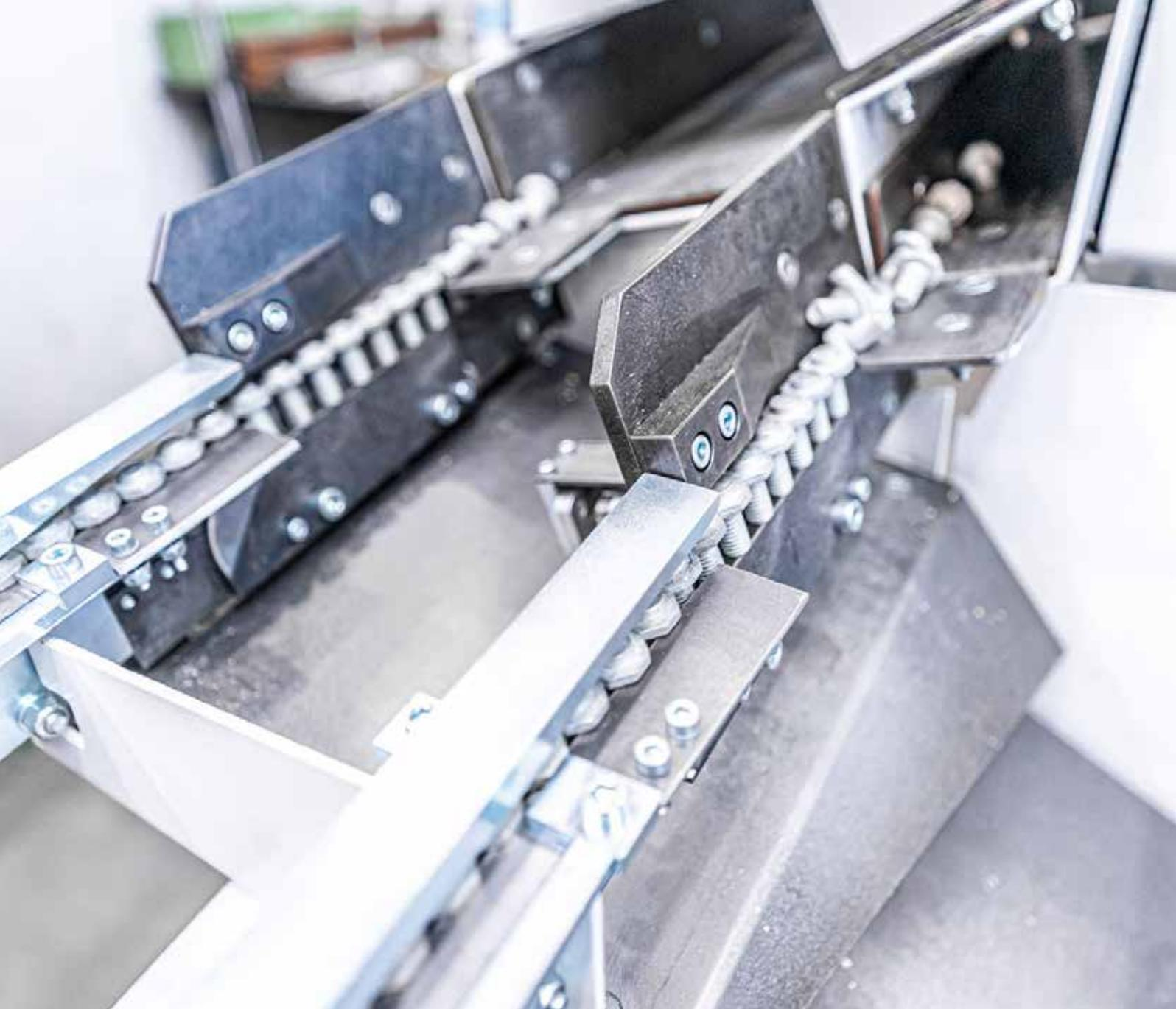
rejected by the linear feeder and are recirculated to the storage container. The sorting feeders are equipped with pneumatic deflectors to prevent the magazine from overflowing and to control the feeding lane in case a screw is left out.
