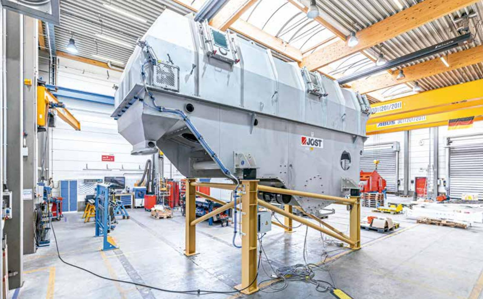
a heat exchanger. This design results in an energy efficient operation whilst maintaining as much flexibility as possible for different product types. A screen following the dryer separates the material stream into three grain sizes. Furthermore, the entire equipment is noise and heat isolated.
