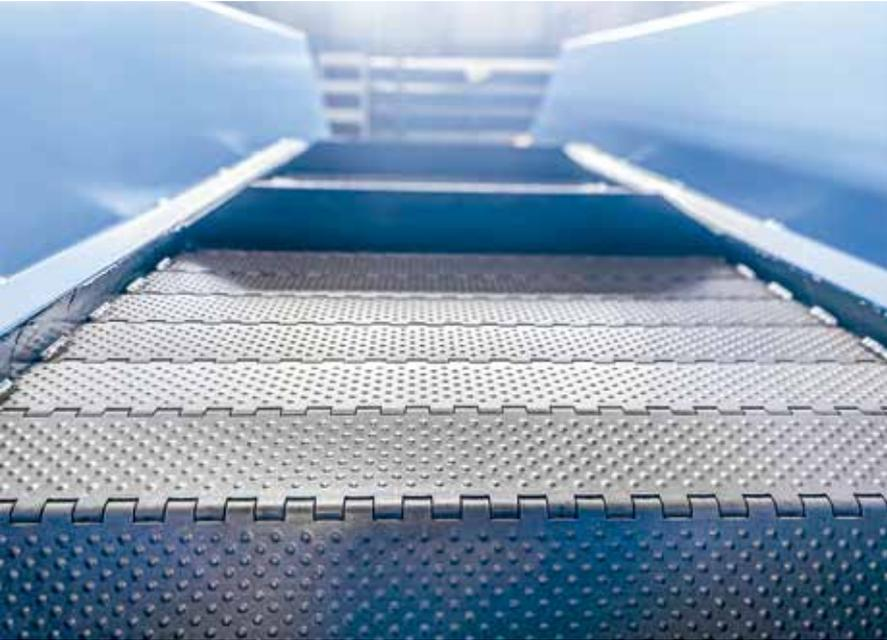
The objective here was to sort and dispose aluminum and steel scrap from a total of six steel presses. GOESSLING designed and manufactured eight Hinged Belt Conveyors with a combined length of 130 meters, a partition of 125 mm and an effective width of 1,025 mm.
