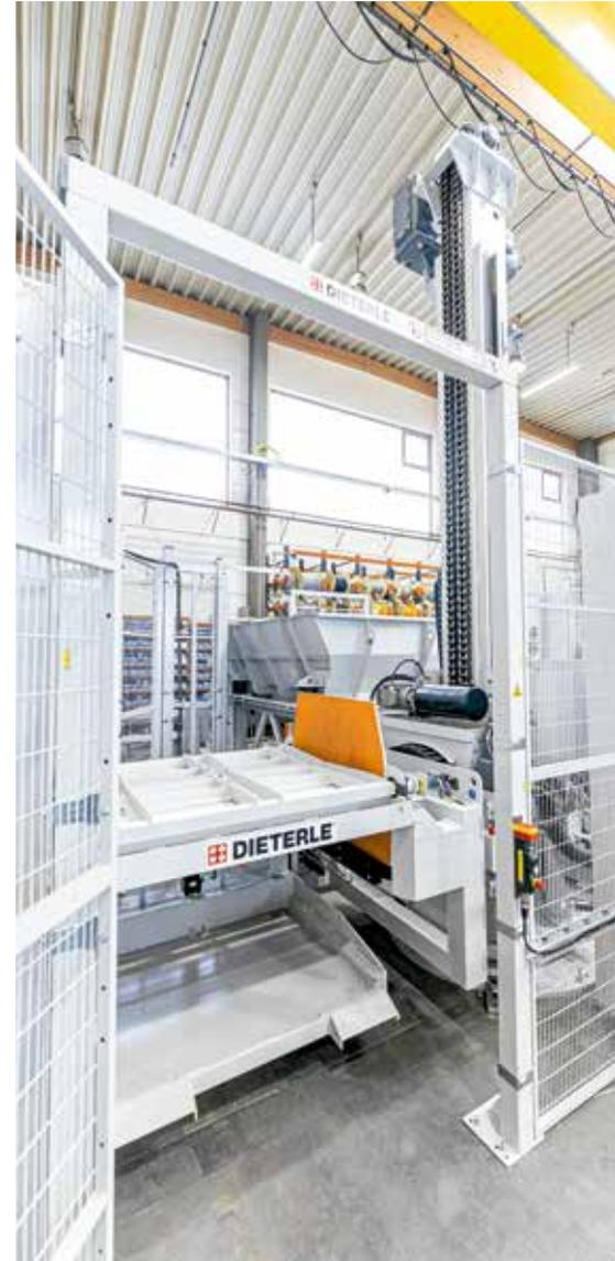
in the feeders, individually programmed SPS formulations for different parts and the “dipping” motion into the feeder. Furthermore, the JOEST Feeders are equipped with the latest JM-8 Magnetic Drive which stands out due to its low noise emissions and optimal dosing performance.
